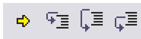
Figure 2. The Debug Buttons: Show Current Statement, Step In, Step Over, Step Out.
